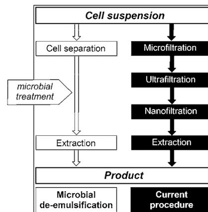
**Figure 3.** Comparison of current workup technology and the simplification accomplished by microbial de-emulsification.
